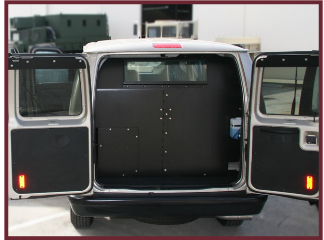
COMPLETED RHINO SHUTTLE™ – REAR WALL ARMORING
